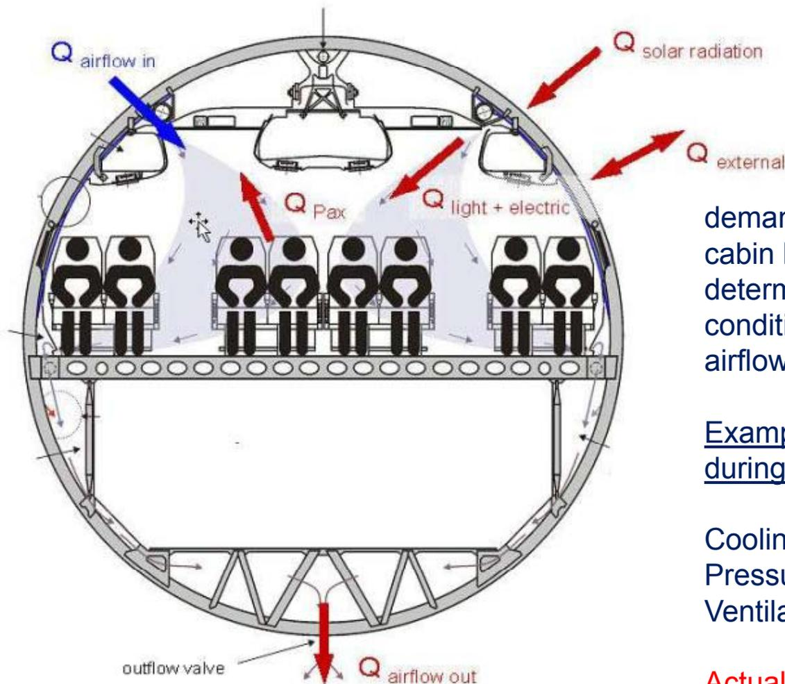
demand of cooling airflow based on cabin heat balance and air exchange determines performance of air conditioning (above minimum certified airflows) and pressurization.
