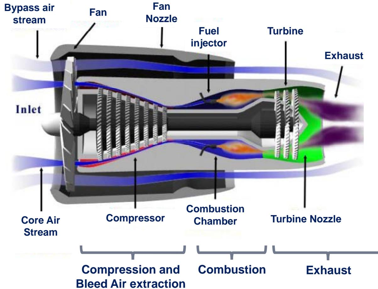
**Air is taken from compressor stage UPSTREAM of the combustion chamber**
