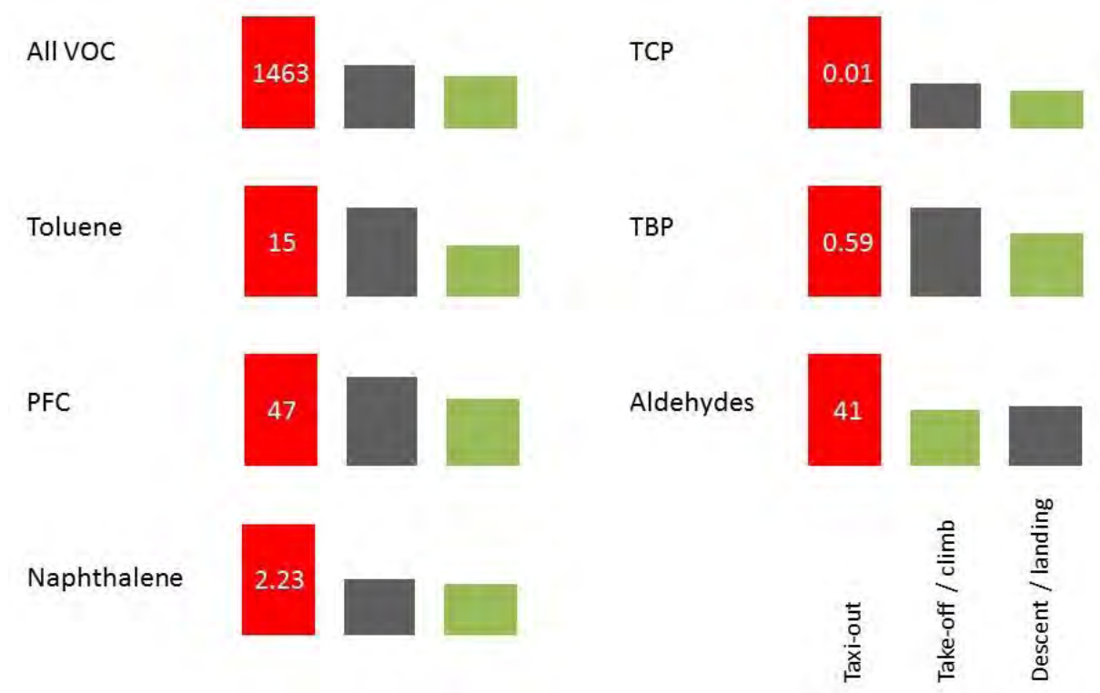
Figure 52 Observed uniform course of the quantitative contaminant data from the Main study (bleed air supply) with respect to the investigated flight phases. The individual concentrations in the pictograms are given in a colour code (high = red, medium = grey, low = green). For the take-off values the concentrations in \mu\text{g}/\text{m}^3 are additionally given (median values in white numbers) for comparability reasons. Note that the outcome is totally consistent although different methodologies were used for VOC, OPC and aldehyde detection. The compound selection focuses, with exception of TCP (normally detected in concentrations far below 0.01 \mu\text{g}/\text{m}^3 ), on contaminants representative for the aircraft cabins. However, almost all detected cabin VOC follow this concentration course. An opposing trend was found for discontinuous release only. The white number given in the bar for all VOC represent the sum of all VOC ( \mu\text{g}/\text{m}^3 ) measured during the taxi-out flight phase. These values are also given for all other presented contaminants. In case of toluene (commonly known indoor contaminant), perfluorinated compounds (PFC; air condition), naphthalene (mothballs), TBP (aircraft hydraulic oil) and short-chain aldehydes (interior, adhesive, etc.) an origin from engines are not considered to be very likely. Solely TCP is supposed to be related to undesired engine oil entry and serves, therefore, as a marker for bleed air contaminations.
