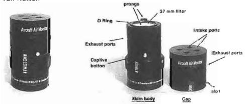
The assembled sampler
