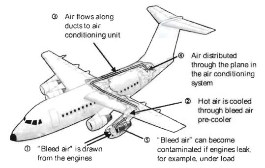
One further feature is that the ducting for the latter part of the air conditioning system is partially made of fibre glass, probably used for weight purposes. However, oil leaking through the system will adsorb onto and into fibre glass materials, and even if removed from ducting, will continue to vapourise from such surfaces. This perhaps provides a reason for the "146 smell".
