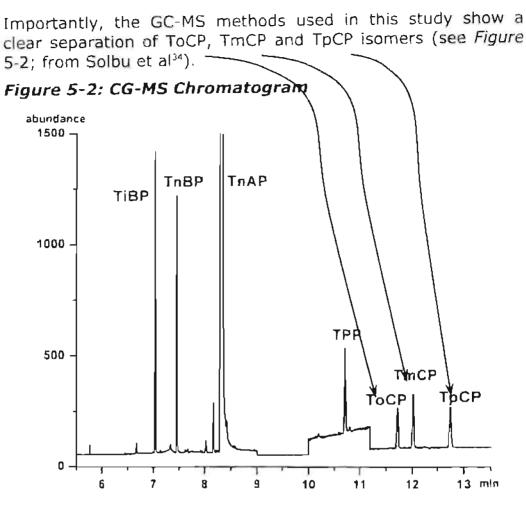
Fig. 2. GC-MS (SIM) chromatogram from splitless injection of 30 pg TiBP, TnBP, TPP ToCP, TmCP and TpCP and 3 ng volumetric internal standard (TnAP). The organophosphates were separated on a VF-5ms CP8957 capillary column (30 m × 0.32 mm,  $d_f = 1.00 \,\mu$ m) with a carrier gas flow rate at 3.5 mL/min. The GC-oven temperature was 40-320 °C during a total time of 14 min. Injector temperature was set to 280 °C.
